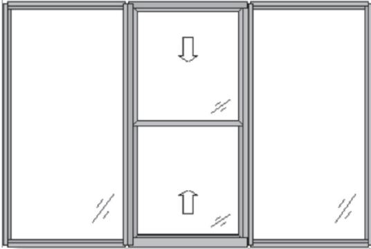
All Carinya double hung window sashes feature corner blocks in all four corners of the sashes. These blocks make the sash more rigid, reducing twist and movement. This reduction in movement increases the performance of the window by reducing opportunities for air, water and dust infiltration.
